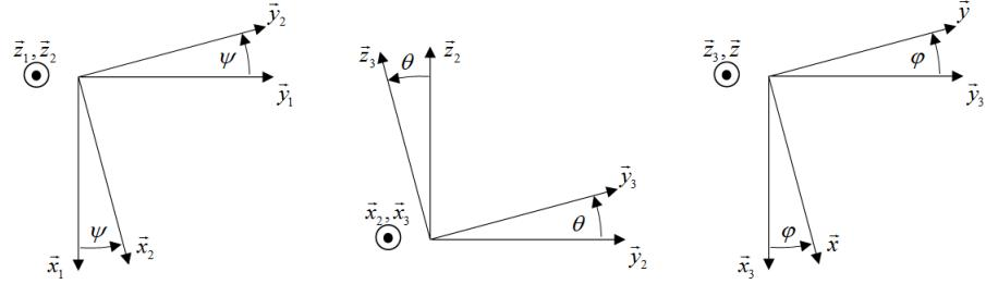
$$(\vec{x}_1, \vec{y}_1, \vec{z}_1) \xrightarrow{\text{rot}(\vec{z}_1, \psi)} (\vec{x}_2, \vec{y}_2, \vec{z}_{1,2}) \xrightarrow{\text{rot}(\vec{x}_2, \theta)} (\vec{x}_{2,3}, \vec{y}_3, \vec{z}_3) \xrightarrow{\text{rot}(\vec{z}_3, \phi)} (\vec{x}, \vec{y}, \vec{z}_{3,3})$$
